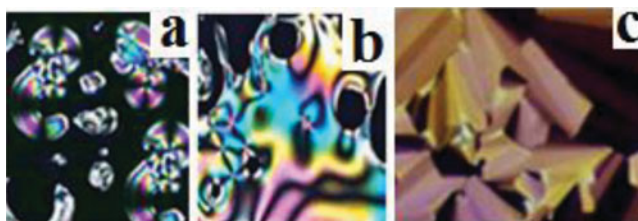
Figure 2. Microphotographs obtained in between the crossed polars, (a) coexistent biphasic region of nematic ( \text{N} + \text{I} ) phase (250 \times ). (b) Lyotropic nematic ( \text{N}_\text{D} ) phase (250 \times ). (c) Smectic-G phase (250 \times ).
